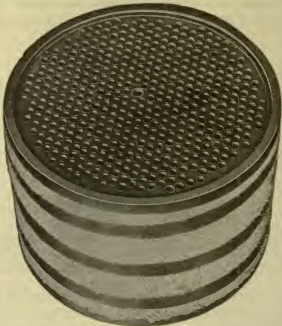
FIG. 350.—The Stanley fire tube boiler. The shell and lower head are of one piece of pressed steel. The bands, as shown in the cut are of thin brass, to hold the asbestos covering in place.
